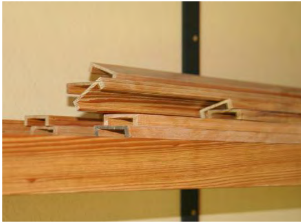
Dado cut bracket caps are cut from solid stock.
