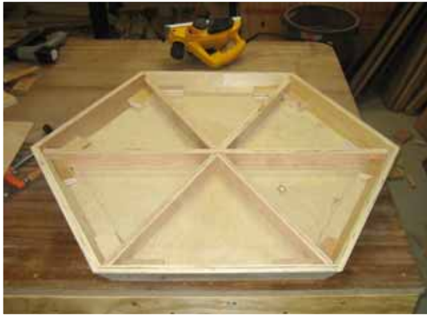
Inner structure of the hexagonal base.
