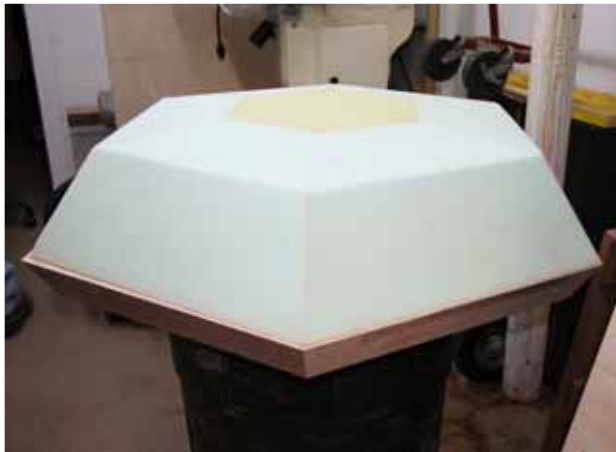
Styrofoam cut to fit the faceted hexagonal form.
