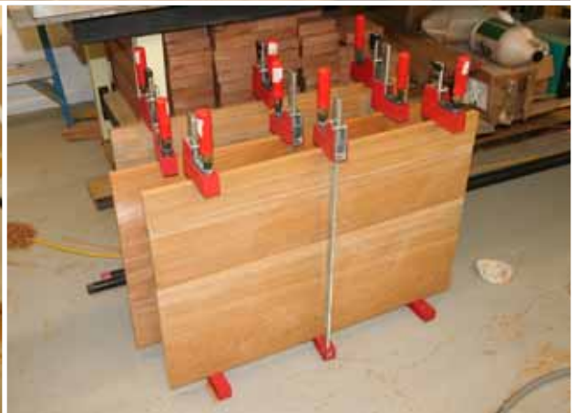
Solid cabinet sides are built-up from smaller planks.
